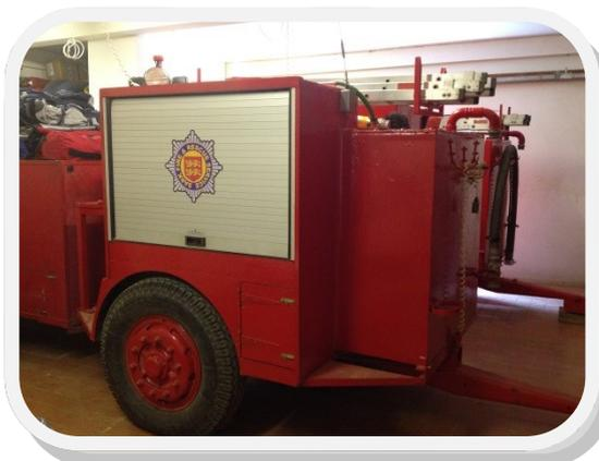
The basic design of the appliances has not changed since 1958, although now the equipment is stowed on board in closed lockers. Each appliance has a Hale HP200 pump which gives a maximum flow of 852 l/pm, along with one hose reel, eight lengths of 45 mm hose, one length of 75 mm hose, various branches and hand tools. The first appliance carries, in addition, a Tetra radio Repeater/Gateway which links 4 handhelds with Guernsey
